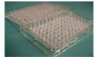
MBEC lid fits into a 96-well microtiter plate
